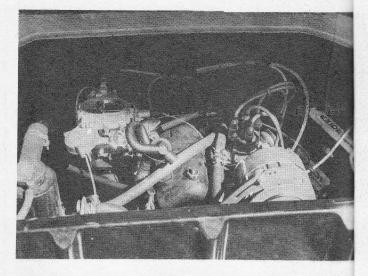
Engine is directly behind the cockpit with a luggage locker behind it. Most of the engine is quite accessible, but with the extra long cables from front to rear everything needs to be spoton for operation of clutch and accelerator.
