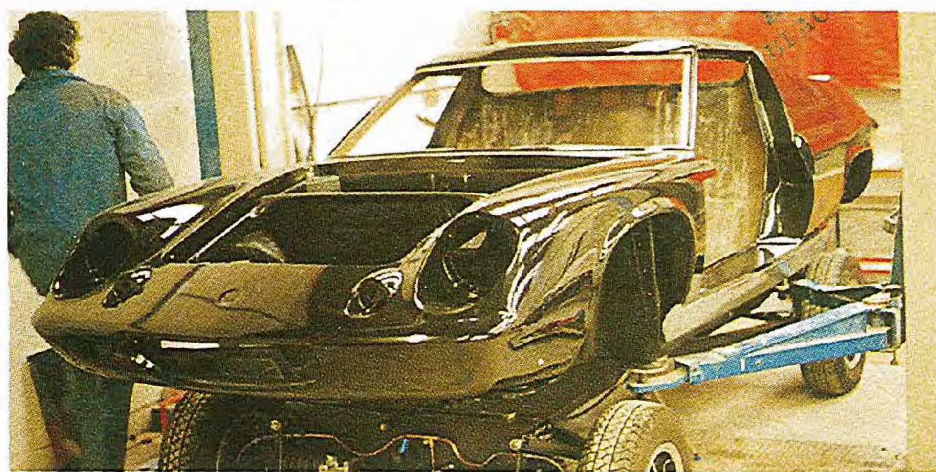
Damage to glassfibre body ground out and relaminated
