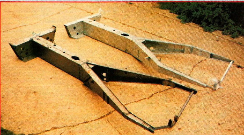
The two Europa chassis. The one nearest the camera is for the Renault-engined car and is fabricated by Fibreglass Services, the one behind it comes from Lotus for the TC cars. The differences are slight but crucial.
